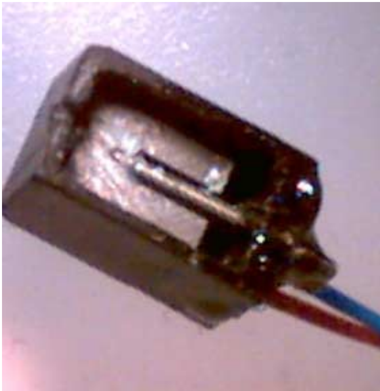
Piezo-bender prototyped for "in-tire" sensor network
